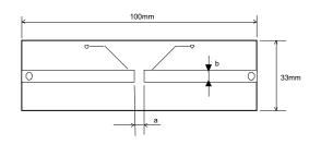
Glass epoxy body on one side Board thickness : 1.6 mm
