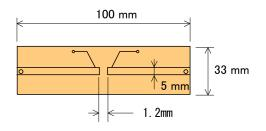
Glass epoxy on one side Board thickness : 1.6 mm Copper layer : 35μm
