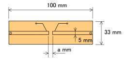
Glass epoxy on one side Board thickness : 1.6 mm Copper layer :  $35\mu m$
